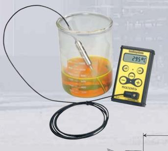
The HERMetic Onecal can also be used in laboratories for verification of existing temperature measuring equipment. The high accuracy of this thermometer allows a reliable temperature reading. The HERMetic Onecal can be supplied without frame and with a 2 m / 7 ft cable. This type of unit can very well be used for temperature verification anywhere in a laboratory or on a railtrain tank if the opening is bigger than 16 mm / 5/8" in order to allow the penetration of the sensor.
