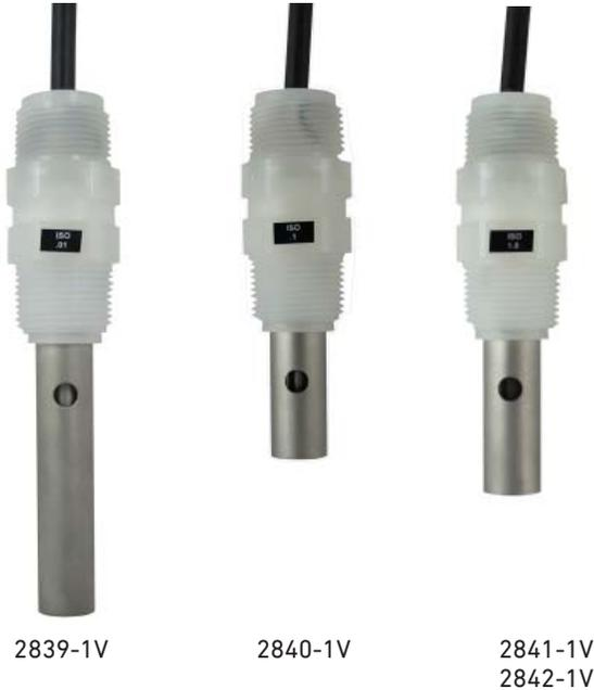
The Signet 2839-1V(D) to 2842-1V(D) Conductivity/Resistivity Electrodes are available in four cell constants from  $0.01$  to  $10.0 \text{ cm}^{-1}$ , and are suitable for a wide variety of applications from high purity water quality monitoring to weak acids and bases. 316 SS electrode surface finishes are controlled in a precision bead blasting operation to ensure measurement accuracy and repeatability.
